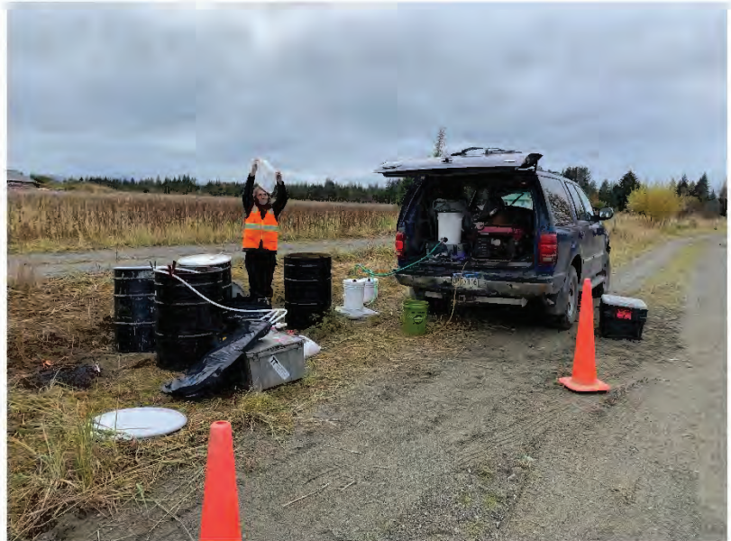
Exhibit 2-2: Monitoring well development; visually checking turbidity.
